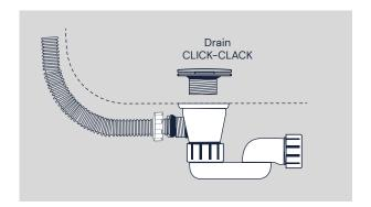
WARNING, BEFORE CONNECTION AND DEFINITIVE INSTALLATION OF THE BATH: Build or install the necessary support, then check the correct seating of the bathtub on it, if everything is correct, proceed to make the connections and to the final positioning of the bathtub.
