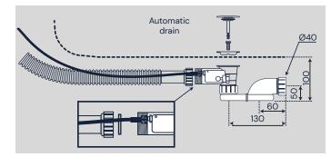
WARNING, BEFORE CONNECTION AND DEFINITIVE INSTALLATION OF THE BATH: Build or install the necessary support, then check the correct seating of the bathtub on it, if everything is correct, proceed to make the connections and to the final positioning of the bathtub.
