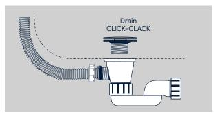
WARNING, BEFORE CONNECTION AND DEFINITIVE INSTALLATION OF THE BATH: Build or install the necessary supportand then check that the bathtub is correctly seated on it, if everything is correct, proceed to make the connections and to the final positioning of the bathtub.
