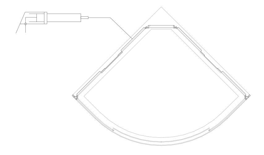
15. Apply silicone. No using within 24 hours.
