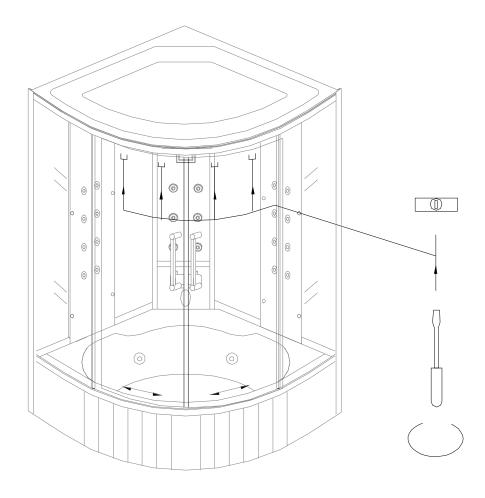
14. Adjust minimum gap between the sliding door use small screwdriver to adjust the screws on the wheels (as illustrated in the picture), to make sure the gap is minimum and the sliding is smooth.
