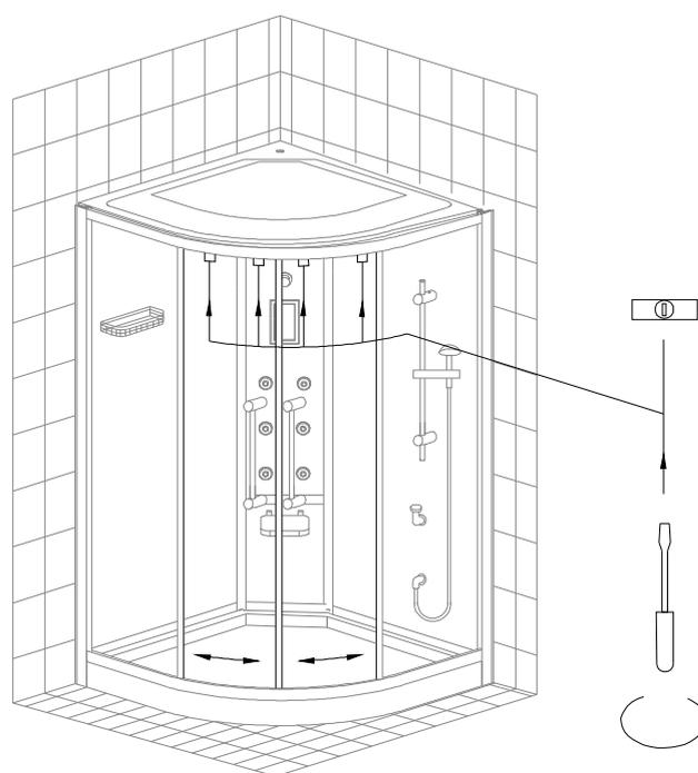
15. Adjust to get minimum gap between the sliding door and the aluminum profile: use small screwdriver to adjust the screws on the wheels (as illustrated in the picture), to make sure the gap is minimum and the sliding is smooth.
